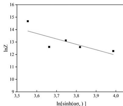
Figure 3 Relation curves of  $\ln Z$  and  $\ln[\sinh(\alpha\sigma_s)]$
