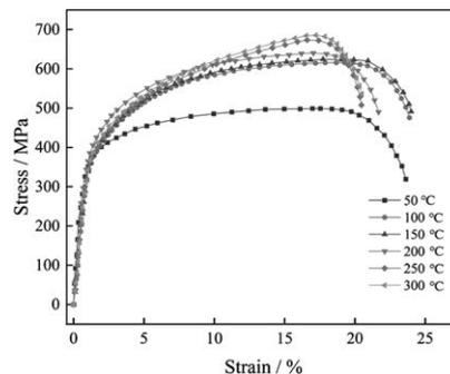
Figure 1 Tensile stress-strain curves under different temperature conditions of low carbon alloy steel
