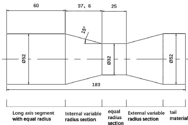
Figure 2 Test piece of hollow axis variable diameter section
