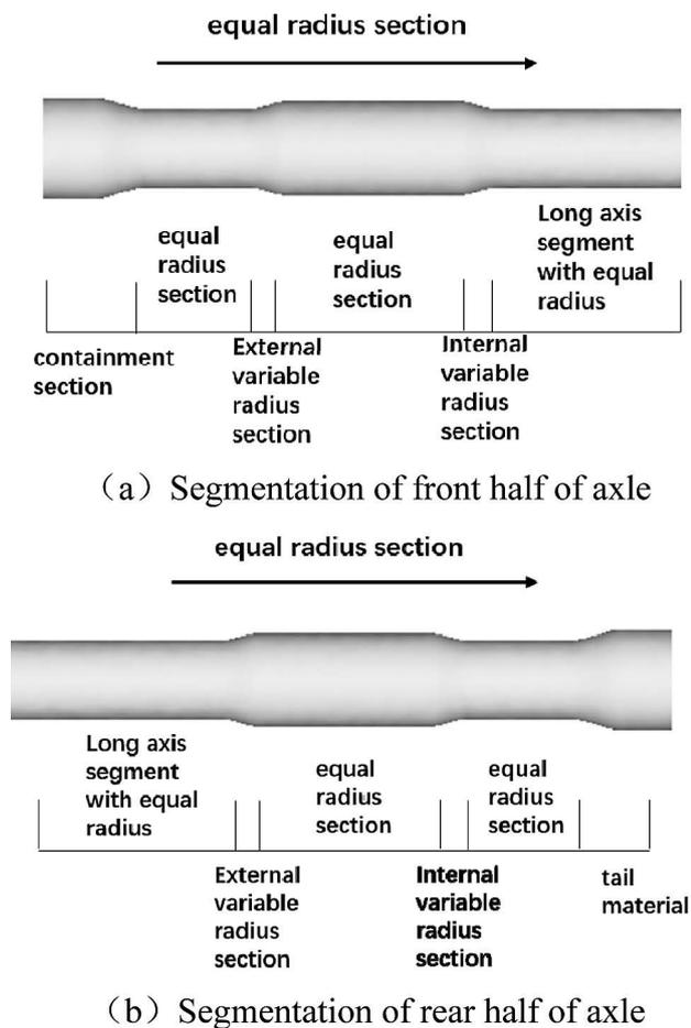
Figure 1 Segmentation of hollow axis
