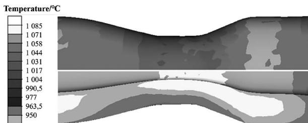
**Figure 4** Temperature field distribution in the equal diameter section
