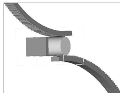
**Figure 1** Finite element rolling model of gear cross wedge rolling
