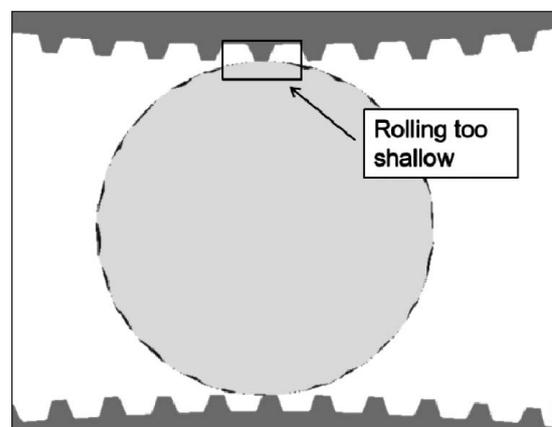
Figure 3 Rolling Process of Test 1
