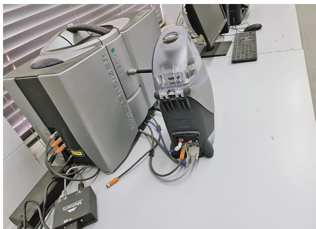
Figure 1. Mastersizer 3000 instrument (Yanbu Cement Company Lab, KSA)
