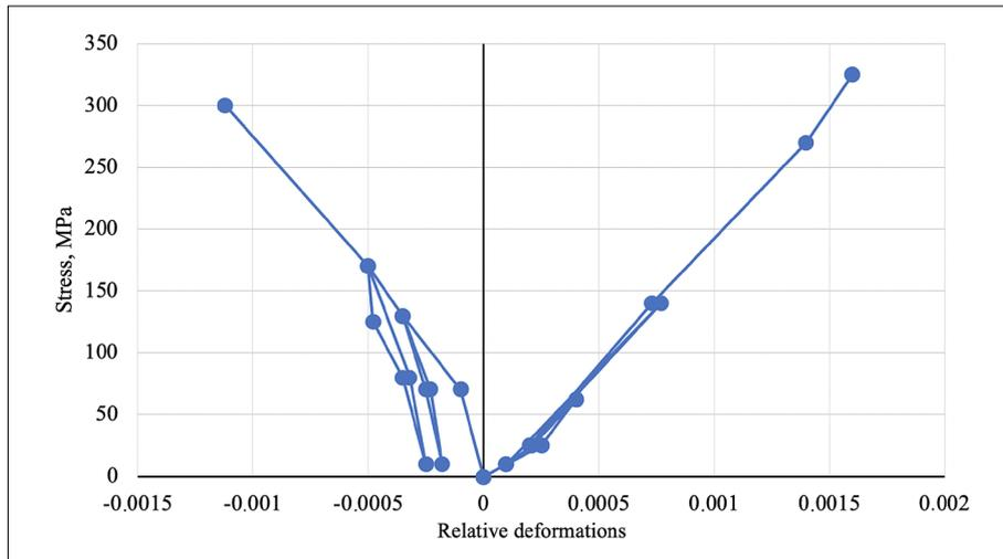
**Figure 4:** Uniaxial rock compression perpendicular to stratification
