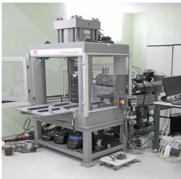
**Figure 2:** MTS816 rock mechanics experimental system
