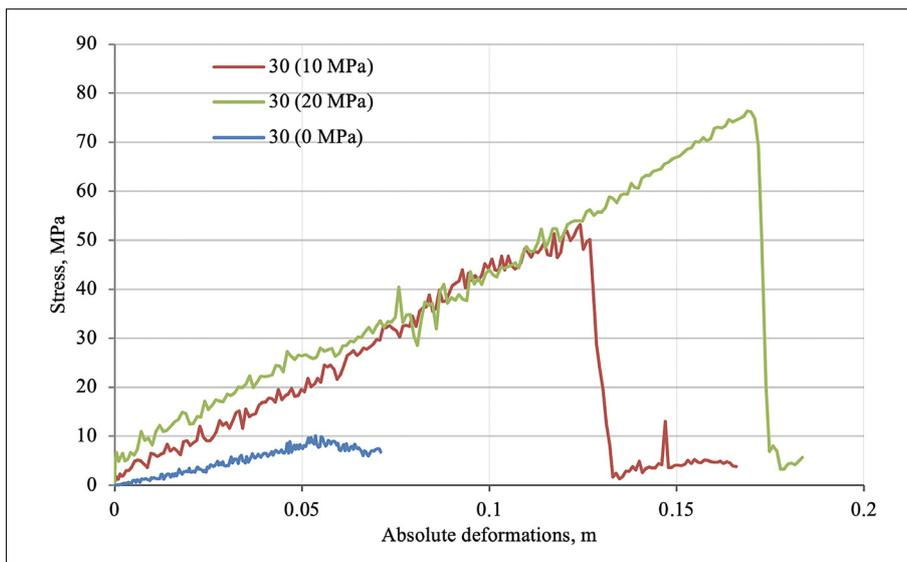
**Figure 10:** Tests of the jointed rock mass in 3D stress state at a 30° inclination angle of the main joint pattern
