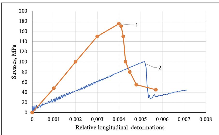
**Figure 16:** A comparison of compression tests of a hard rock sample (1) and a jointed granite rock mass at 90° of the joint pattern inclination (2)
