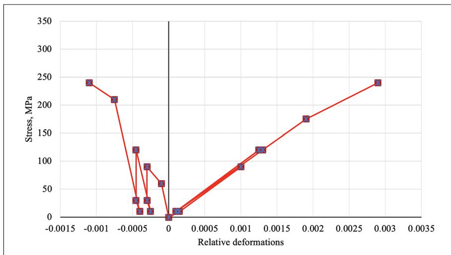
**Figure 5:** Uniaxial rock compression parallel to stratification
