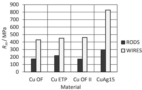
**Figure 2** Comparison of ultimate tensile strength of rods and wires presented materials including: oxygen free copper Cu-OF, Cu ETP, oxygen-free copper Cu OF II and CuAg15 alloy
