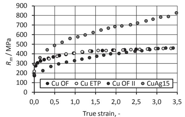
**Figure 4** Strengthening curve of wires of oxygen free copper - Cu OF, Cu ETP, oxygen-free copper - Cu OF II and CuAg15 alloy
