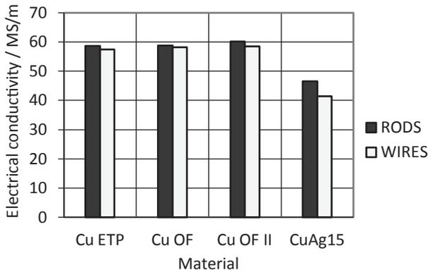
**Figure 1** Electrical conductivity in %IACS of rods and wires of presented materials like: oxygen free copper Cu-OF, Cu ETP, copper from recycling technology Cu OF II and CuAg15 alloy
