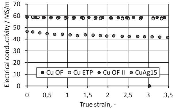
**Figure 3** Change of electrical conductivity as a function of true strain of wires of various materials: oxygen free copper Cu-OF, Cu ETP, copper from recycling technology Cu OF II and CuAg15 alloy
