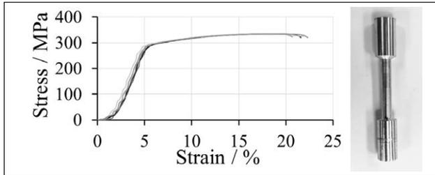
**Figure 4** Stress-strain curve of EN AW-6082 alloy in T6 temper
