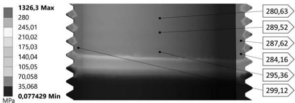
**Figure 5** Exemplary results of FEM analysis (stress pattern) for various wall thickness (Variants 2 and 4)
