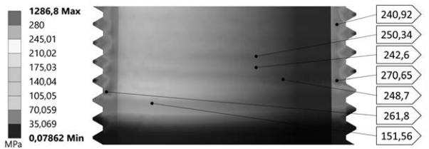
**Figure 6** Exemplary results of FEM analysis (stress pattern) for various taper of the walls (Variants 3, 7 and 8)
