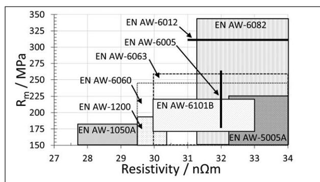
**Figure 2** Mechanical and electrical properties map of the wrought Al alloys
