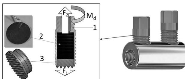
**Figure 1** Screw type connection system and load distribution in clamping unit (screw) during screwing. 1 - screw body; 2 - load and current carrying discs; 3 - screw tip
