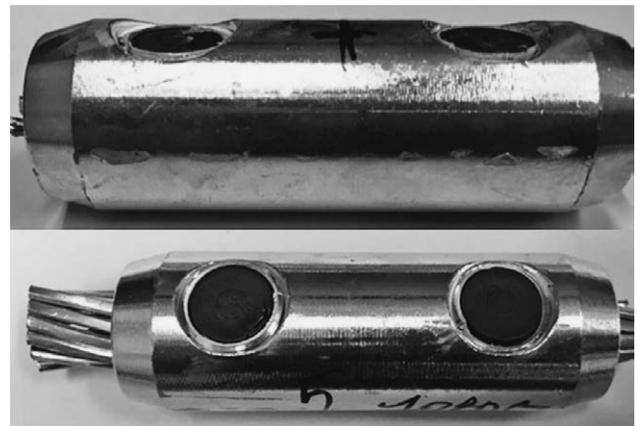
**Figure 7** Connectors with sheared bolts (geometry according to variant #4)
