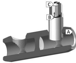
**Figure 3** A model subjected to FEM analysis with boundary conditions
