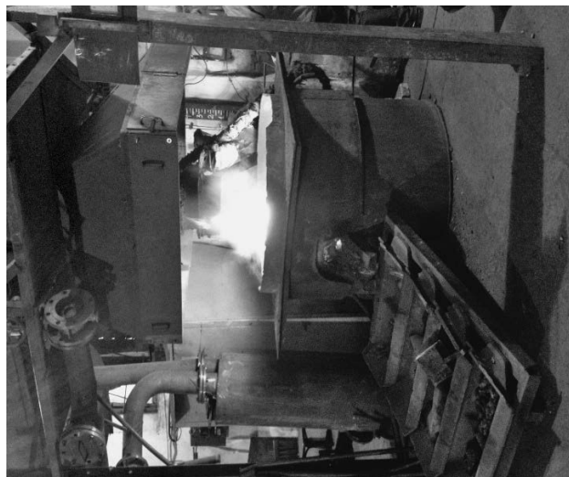
Figure 1 The process of smelting a carbon ferrochrome in an ore-thermal furnace with a transformer capacity of 200 kV·A
