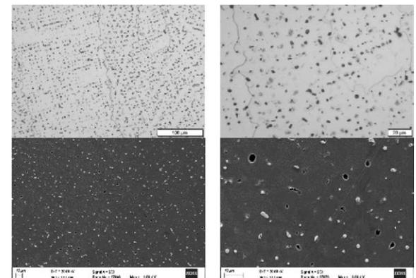
Figure 9 The microstructure on the rod cross-section - the end of the casting process
