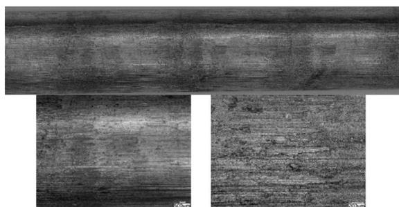
**Figure 11** Surface analysis of a continuously cast rod - the end of the casting process
