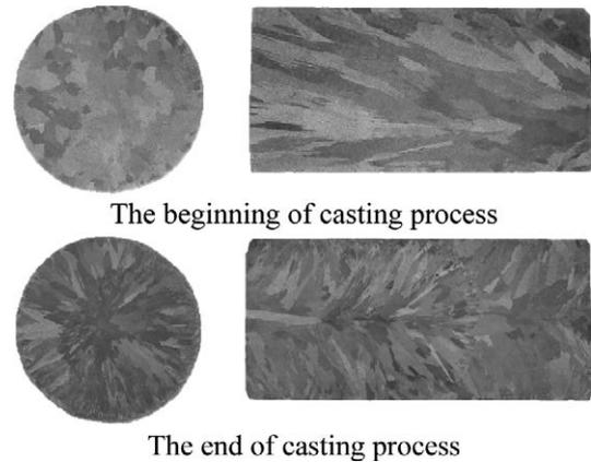
Figure 7 The macrostructure of continuously cast rods
