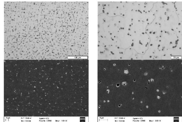
Figure 8 The microstructure on the rod cross-section - the beginning of the casting process
