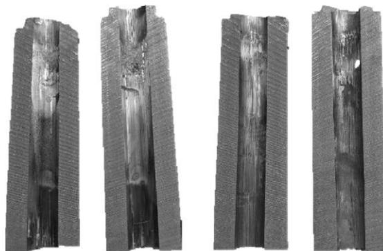
Figure 2 View of the cross-section of strands 1 and 2 of the R4550 grade crystallizer
