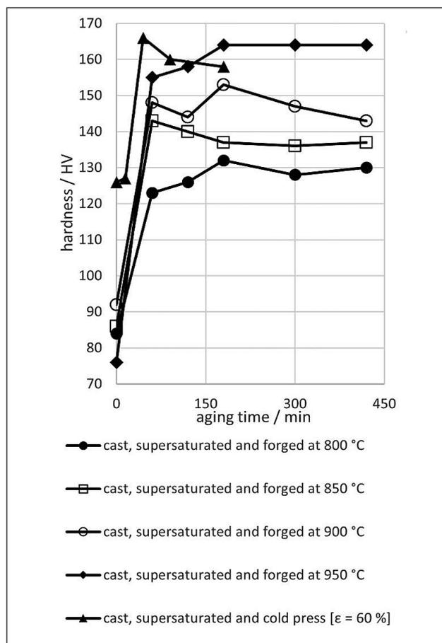
**Figure 5** The influence of aging time on the hardness of pressed CuCrTiAl alloy.
