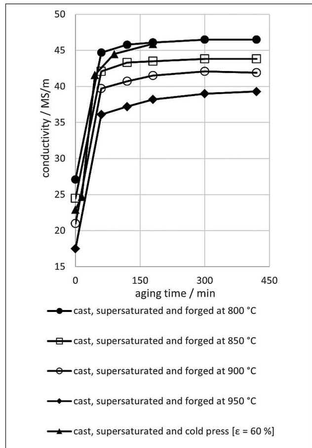
**Figure 4** The influence of aging time on the conductivity of pressed CuCrTiAl alloy
