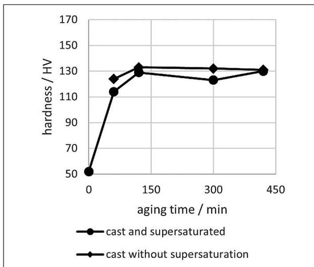
**Figure 3** The influence of aging time on the hardness of cast CuCrTiAl alloy.
