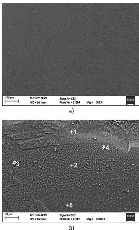
**Figure 6** Microstructure and EDS analysis of the CuCrTiAl alloy after hot deformation and aging at 480 °C for 2 hours, where the individual points have the following chemical composition (wt. %): 1. Cu-97,8, Cr-2,1, Al-0,1; 2. Cu-99,4, Cr-0,6; 3. Cu-5,1, Cr-82,4, Ti-3,2, P-9,2; 4. Cu-50,8, Cr-2,7, Ti-0,2, Al-26,2, O-20,1; 5. Cu-99,3, Cr-0,6, Al-0,1.
