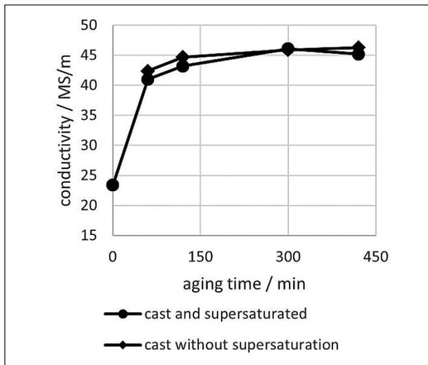
**Figure 2** The influence of aging time on the conductivity of cast CuCrTiAl alloy.
