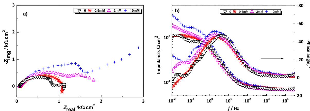
**Figure 11.** Nyquist (a) and Bode (b) plots for AA2024-T3-CFRP galvanic couple immersed for 24 h in 0.05 M NaCl without and with different concentrations of C<sub>2</sub>H<sub>3</sub>N<sub>3</sub>
