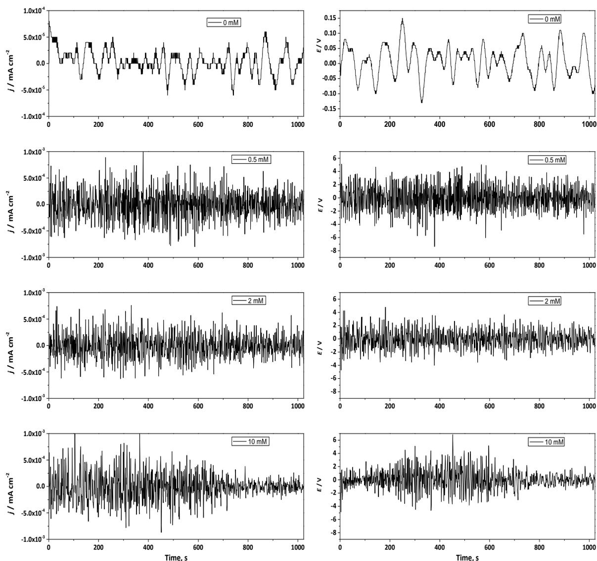
**Figure 7.** Time series of ECN (left) and EPN (right) for AA2024-T3-CFRP in galvanic couple immersed in 0.05 M NaCl without and with 0.5-10 mM  $\text{Ce}(\text{NO}_3)_3 \cdot 6\text{H}_2\text{O}$  at the beginning of the test (1 h)
