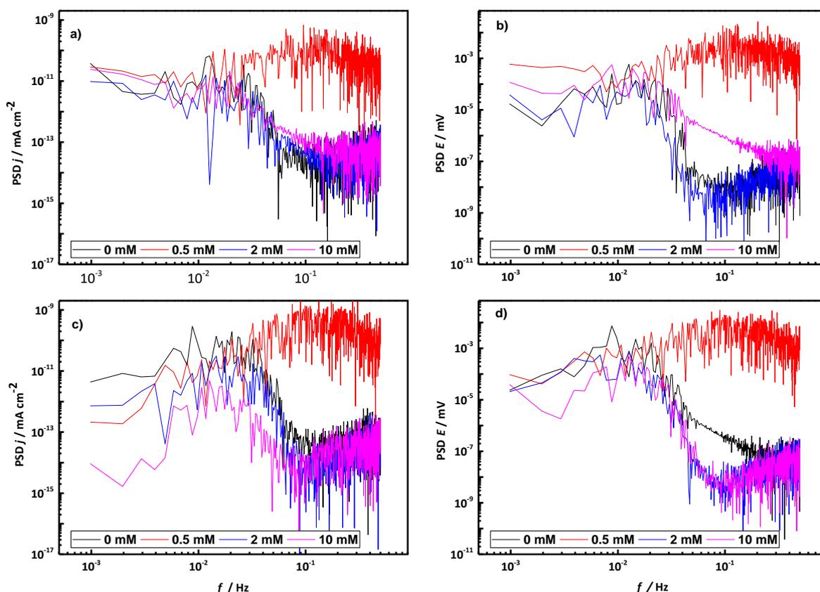
**Figure 6.** PSD plots of current (left) and potential (right) for AA2024-T3-CFPR in galvanic couple immersed in 0.05 M NaCl without and with 0.5-10 mM  $C_2H_3N_3$  at the beginning (a and b) and the end (c and d) of the test
