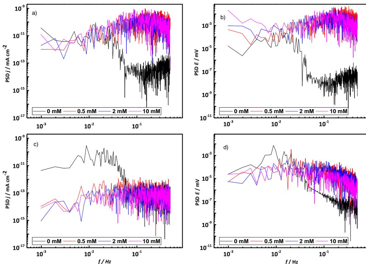
**Figure 10.** PSD of current (left) and potential (right) for AA2024-CFRP in galvanic couple immersed in 0.05 M NaCl without and with 0.5-10 mM Ce(NO<sub>3</sub>)<sub>3</sub>·6H<sub>2</sub>O at the beginning (a and b) and the end (c and d) of test
