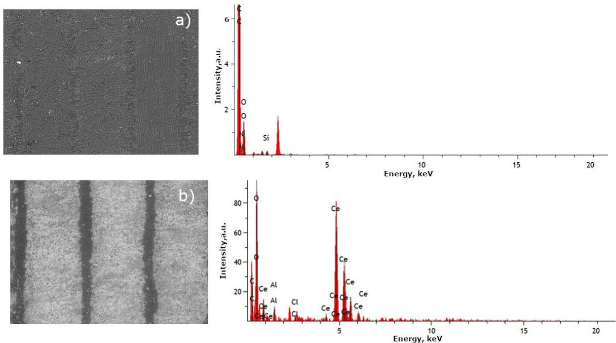
**Figure 20.** SEM micrographs and EDS analysis for CFRP before a) and after b) exposition for 24 h to 0.05 M NaCl with  $Ce(NO_3)_3 \cdot 6H_2O$  as a corrosion inhibitor
