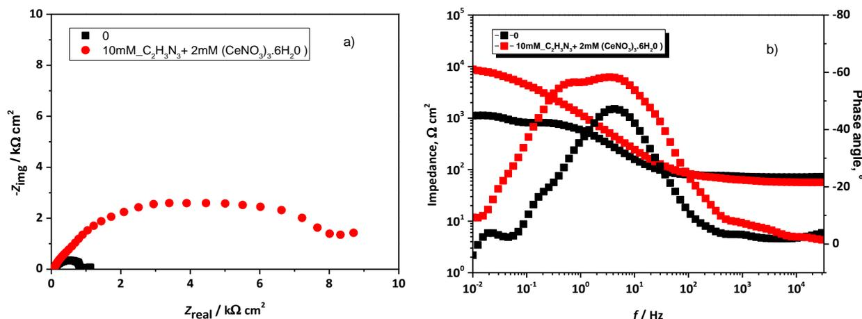
Figure 13. Nyquist (a) and Bode (b) plots for AA2024-T3-CFRP galvanic couple immersed for 24 h in 0.05 M NaCl without and with 10 mM of C<sub>2</sub>H<sub>3</sub>N<sub>3</sub> + 2mM Ce(NO<sub>3</sub>)<sub>3</sub>·6H<sub>2</sub>O
