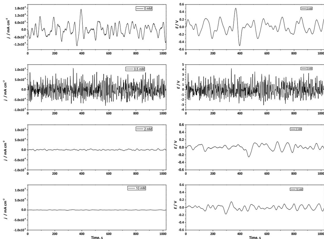
**Figure 4.** Time series of ECN (left) and EPN (right) for AA2024-T3-CFRP in galvanic couple immersed in 0.05 M NaCl without and with 0.5-10 mM  $\text{C}_2\text{H}_3\text{N}_3$  at the end of the test (24 h)
