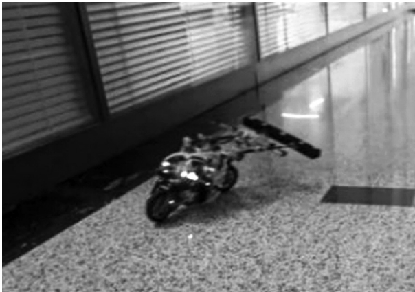
Figure 15. The state of a bicycle that cannot be tilted when turning under control.
