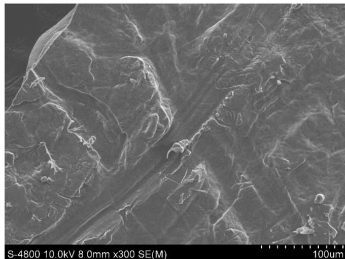
**Figure 2.** Scanning electron microscopy of the dry pectin
