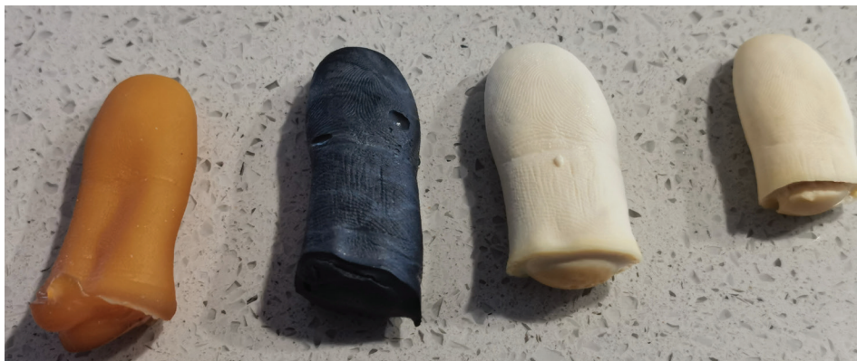
Figure 8 Fabricated fingerprints with alginate mold and latex milk
