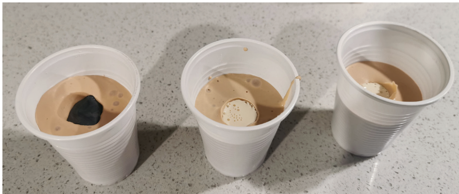
Figure 6 Alginate molds with infused latex milk
