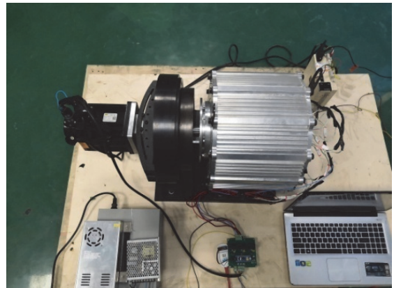
Figure 15 Generator test platform
