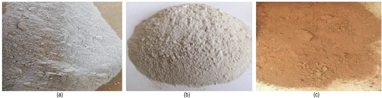
Figure 2 Filler materials: a) CKD; b) GGBFS and c) BP
