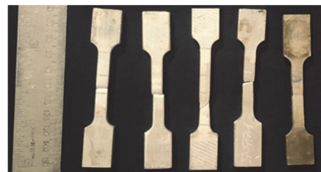
Figure 2 a) Standard tensile specimen as per ASTM E; b) Several specimens after tensile testing
