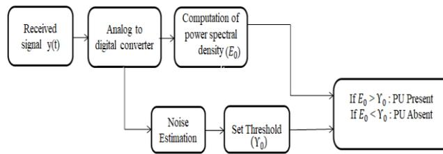
Figure 4. Block Diagram of Energy detector.
