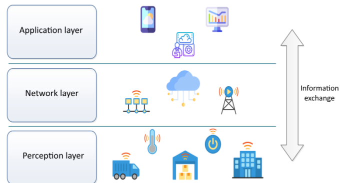
Fig. 1. The three-layer IoT architecture
