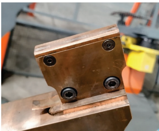
Figure 2 Lower cross-wire welding electrode
