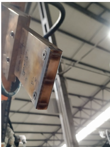
Figure 1 Upper cross-wire welding electrode
