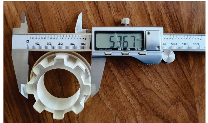
Figure 11 Measurement of the model made by the PolyJet method with the use of a calliper
