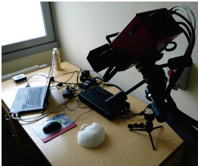
Figure 15 Optical measurement of the skull fragment model made with the 3DP incremental method with the bone defect
