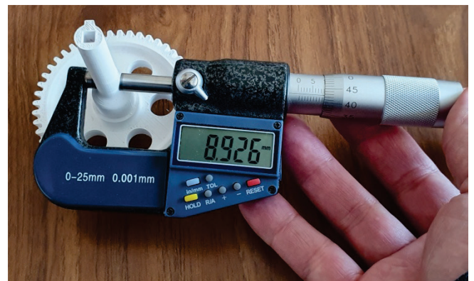
Figure 13 Measurement of the gear model made by the FFF method using a micrometer
