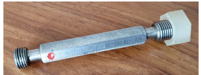
Figure 12 Checking the correctness of the thread geometry of the cap model made using the PolyJet method with the use of a gauge
