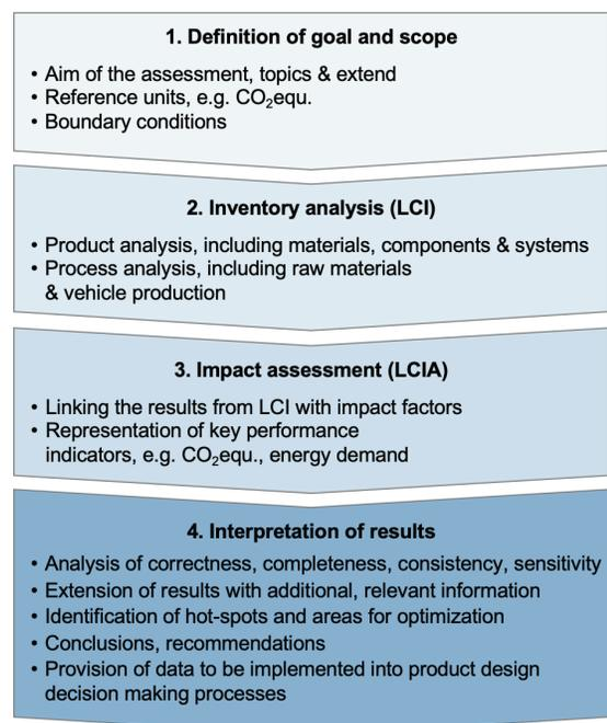
Figure 1 Phases of life cycle assessment (LCA)
