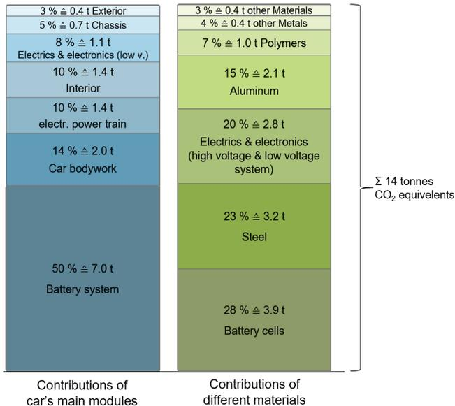
**Figure 4** Contributions of main modules and different materials to CO<sub>2</sub> equivalent emissions of an exemplary electric vehicle production
