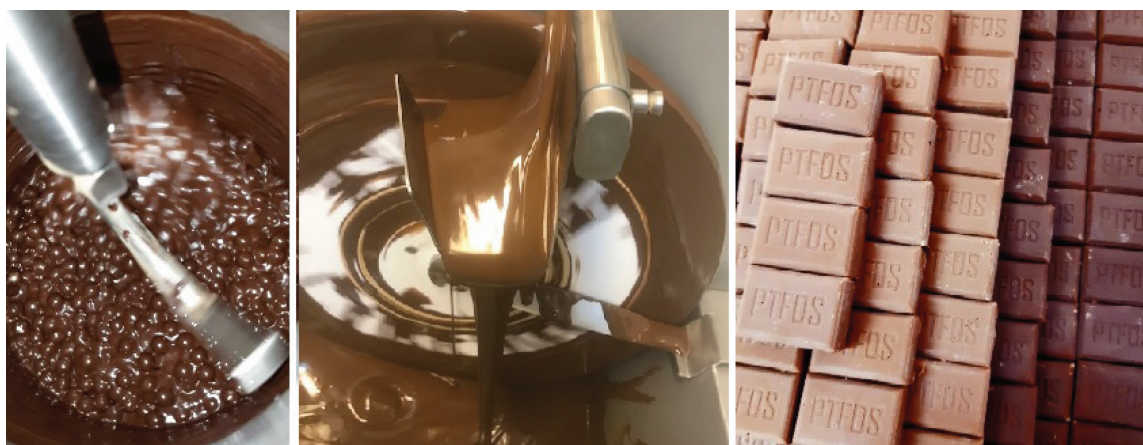
Fig. 6. Laboratory production of chocolate – refining in a ball mill, tempering and moulded chocolate.
