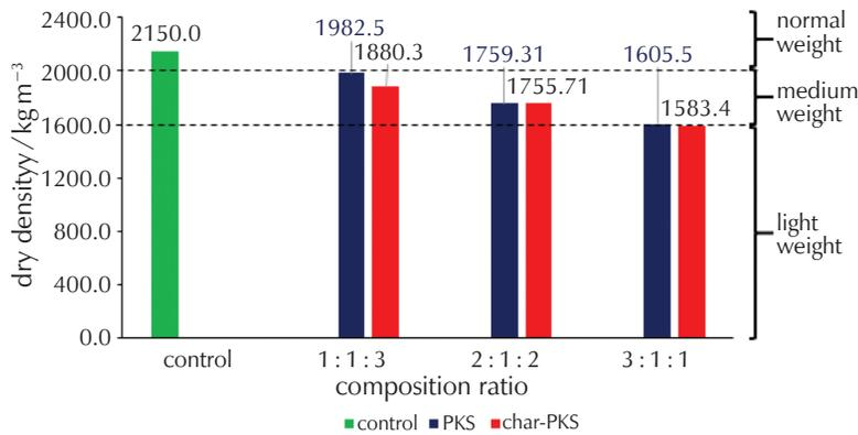
Fig. 8 – Dry density of masonry bricks with different ratios of replacement
