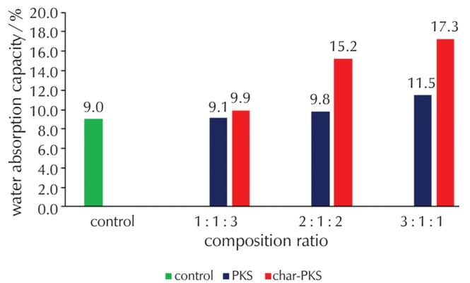
Fig. 7 – Water absorption capacity of masonry bricks with different ratios of replacement
