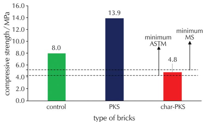
Fig. 4 – Compressive strength of different bricks
