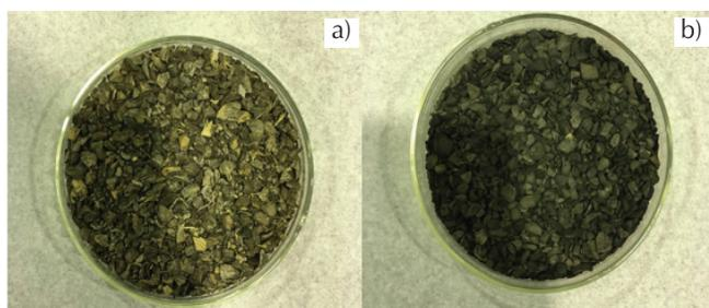
Fig. 2 – PKS (a), and char-PKS (b) used as partial replacement of sand prior to grinding process
