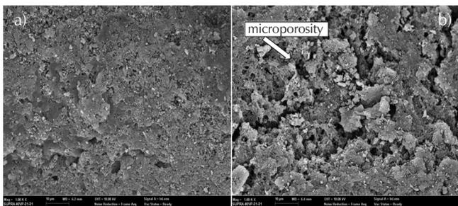
Fig. 6 – FE-SEM image of PKS (a) and char-PKS (b) at 1000× magnification
