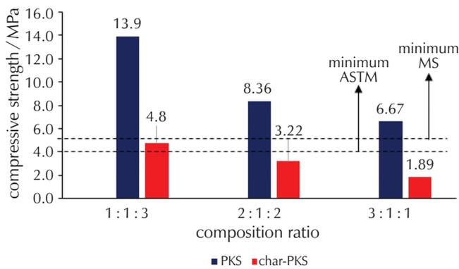
Fig. 5 – Compressive strength of masonry bricks with different ratios of replacement
