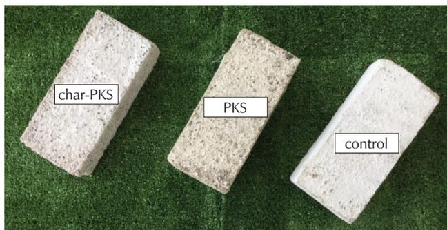
Fig. 3 – Sample of control with PKS and char-PKS bricks of 1 : 1 : 3 composition after 28 days of curing process
