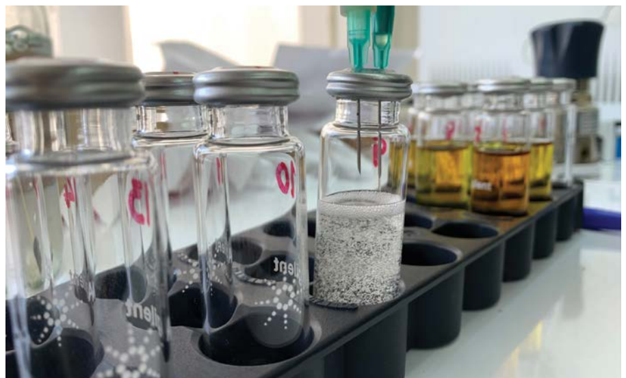
Figure 1. Filling vials according to ASTM D3612
