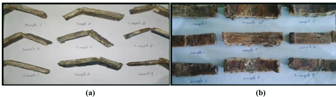
Fig. 3 Composite specimens subjected to tensile strength (a) and flexural strength (b) testing
