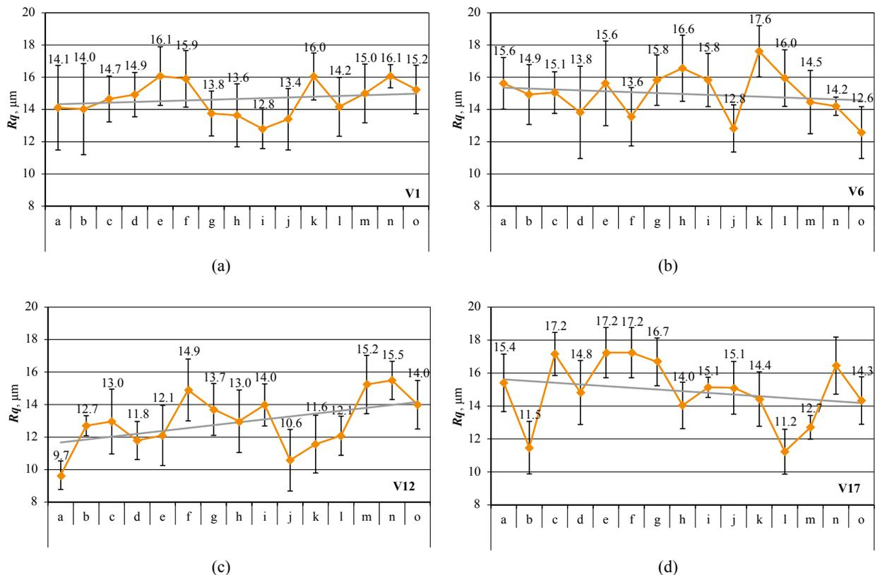
**Figure 6** Progress of  $Rq$  roughness parameter ( $\mu\text{m}$ ) along the stem, measured on typical structure areas, from the canopy to the lowest part of the tree base, on veneers of (a) V1, (b) V6, (c) V12 and (d) V17. The linear trend line is displayed in gray color.
