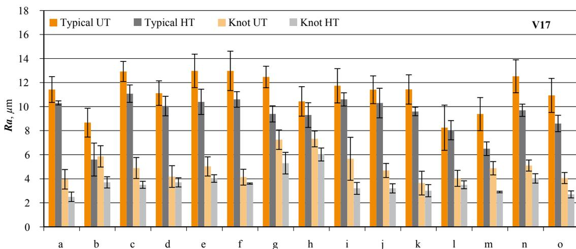
**Figure 13** Mean values ( $\mu\text{m}$ ) and respective standard deviation values of roughness parameter ( $Ra$ ) measured on 15 different points (a-o) along the stem, concerning both knot areas and defect-free areas, on the surface of veneer V17, before (UT- untreated) and after (HT – treated) hydrothermal treatment ( $110\text{ }^{\circ}\text{C}$ -2h)
