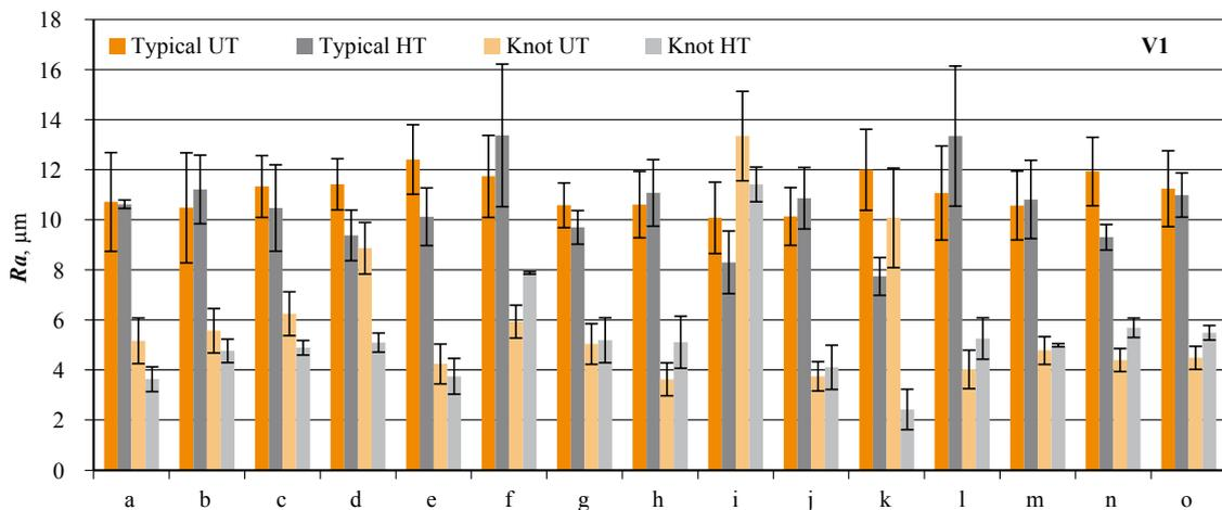
**Figure 10** Mean values ( $\mu\text{m}$ ) and respective standard deviation values of roughness parameter ( $Ra$ ) measured on 15 different points (a-o) along the stem, concerning both knot areas and defect-free areas, on the surface of veneer V1, before (UT- untreated) and after (HT – treated) hydrothermal treatment (130 °C-2h)
