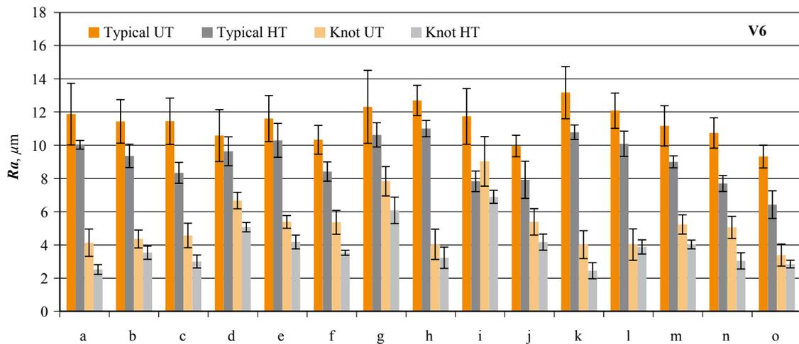
**Figure 12** Mean values ( $\mu\text{m}$ ) and respective standard deviation values of roughness parameter ( $Ra$ ) measured on 15 different points (a-o) along the stem, concerning both knot areas and defect-free areas, on the surface of veneer V6, before (UT- untreated) and after (HT – treated) hydrothermal treatment ( $110\text{ }^{\circ}\text{C}$ -2h)
