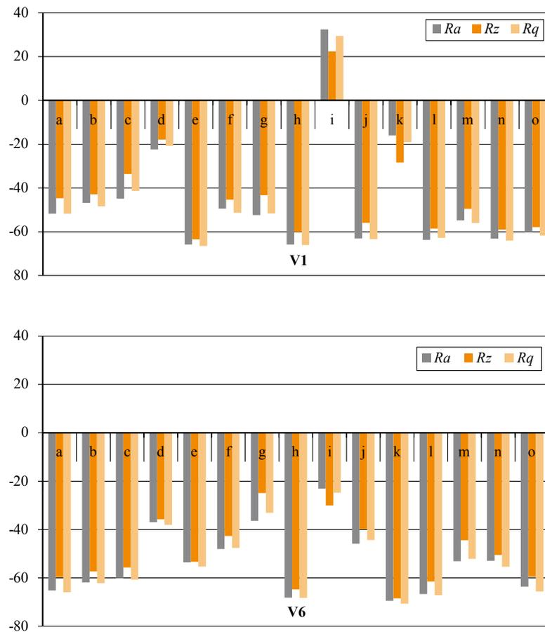
**Figure 8** Percentage values depicting the decrease of roughness parameters (*Ra*, *Rz*, *Rq*) recorded on knot areas (a-o), compared to corresponding areas of non-defect surfaces in veneer V1 and V6
