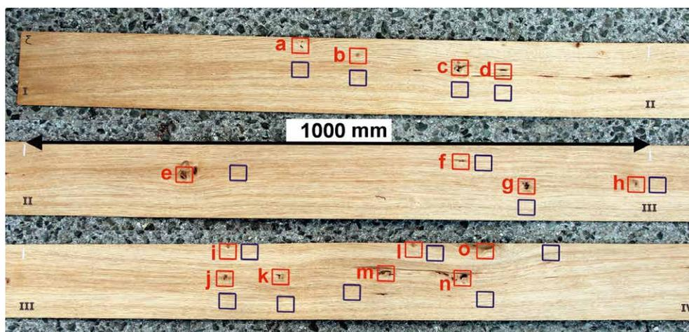
**Figure 1** Distribution of 15 studied knots (a-o) on the surface of veneer sample and configuration of roughness measurement areas ( $30 \text{ mm} \times 30 \text{ mm}$ ) concerning 15 knot areas (red squares), and respective non-defect areas (blue squares)
