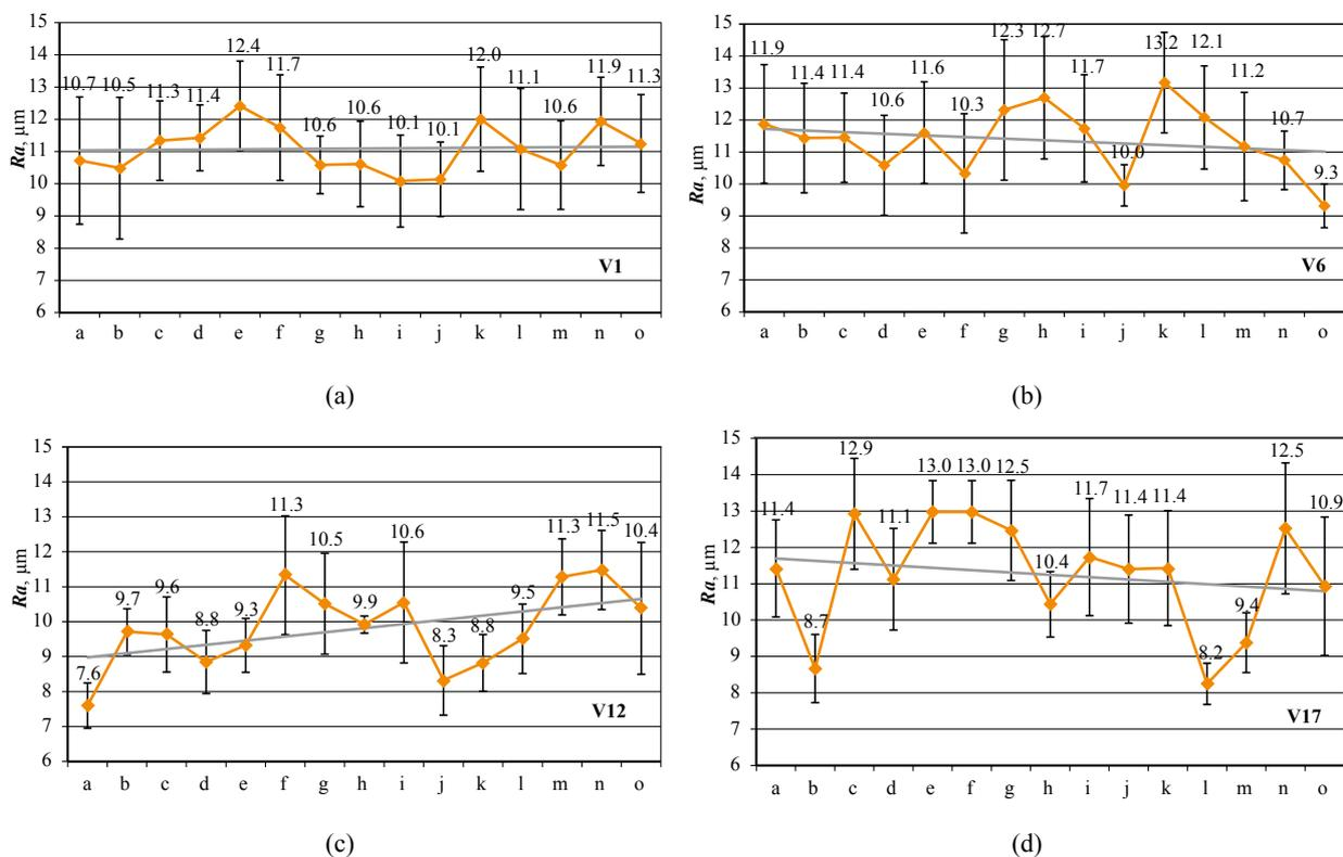
**Figure 4** Progress of  $Ra$  roughness parameter ( $\mu\text{m}$ ) along the stem, measured on typical structure areas, from the canopy to the lowest part of the tree base, on veneers of (a) V1, (b) V6, (c) V12 and (d) V17. The linear trend line is displayed in gray color.
