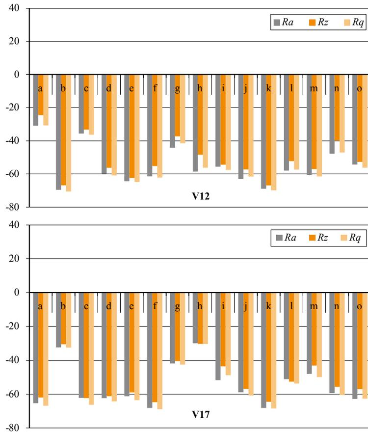
**Figure 9** Percentage values depicting the decrease of roughness parameters ( $Ra$ ,  $Rz$ ,  $Rq$ ) recorded on knot areas (a-o), compared to corresponding areas of non-defect surfaces in veneer V12 and V17
