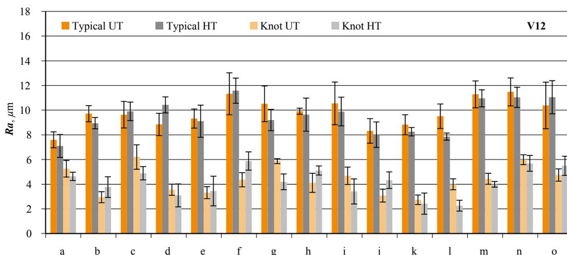
**Figure 11** Mean values ( $\mu\text{m}$ ) and respective standard deviation values of roughness parameter ( $Ra$ ) measured on 15 different points (a-o) along the stem, concerning both knot areas and defect-free areas, on the surface of veneer V12, before (UT- untreated) and after (HT – treated) hydrothermal treatment ( $130\text{ }^{\circ}\text{C}$ -2h)
