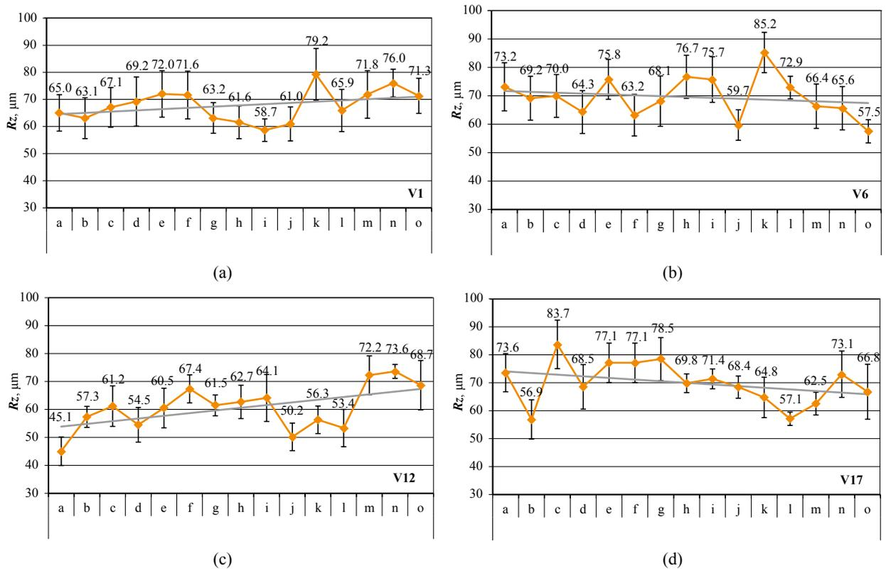
**Figure 5** Progress of  $Rz$  roughness parameter ( $\mu\text{m}$ ) along the stem, measured on typical wood structure areas, from the canopy to the lowest part of the tree base, on veneers of (a) V1, (b) V6, (c) V12 and (d) V17. The linear trend line is displayed in gray color.
