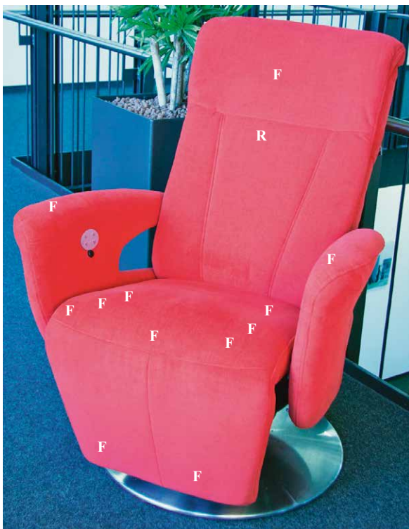
Figure 9 Smart chair with integrated sensors locations (F – FSR, R – radar) (Hesse et al. , 2017)
