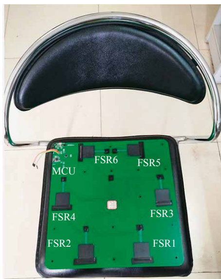
a) Circuit board – front side / Prednja strana
