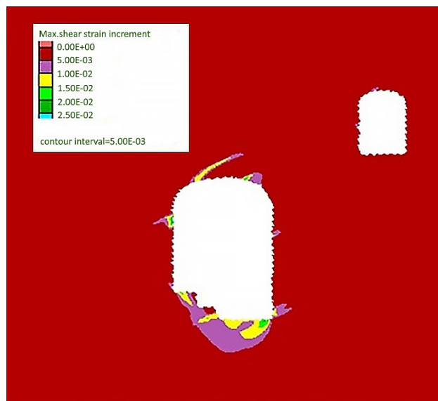
Figure 7: Shear strain ( g_s ) at the roof and sidewalls of the powerhouse and transformer caverns for k=1.893 obtained in this study
