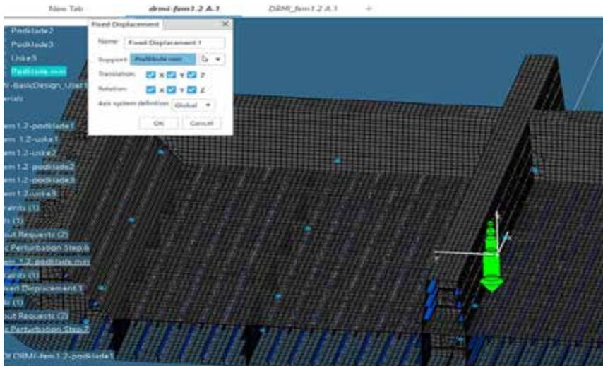
Figure 4: Mesh model representing boundary and loading condition [7].
