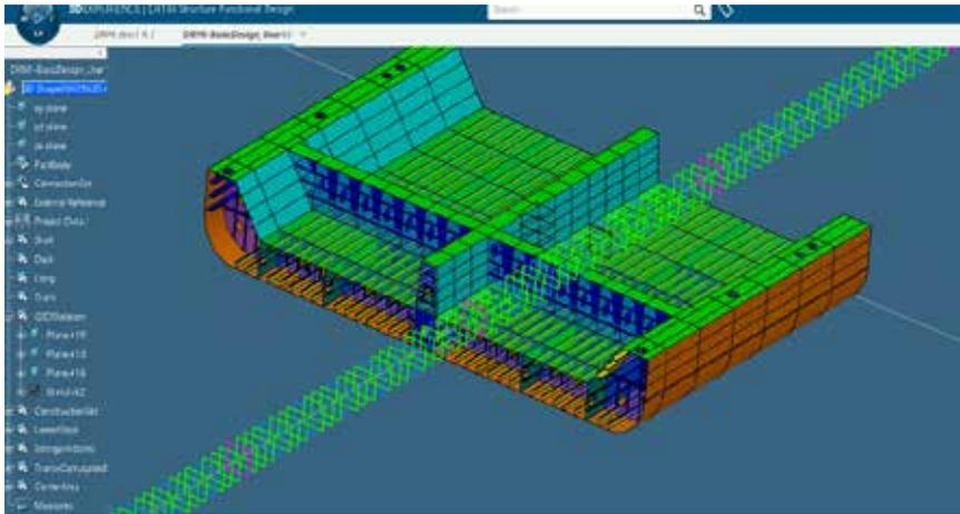
Figure 1: Model of ship double bottom block [7].
