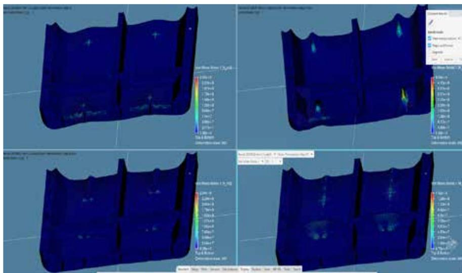
Figure 9: Stress on section for cases 6,7,8 and 10 [6].
