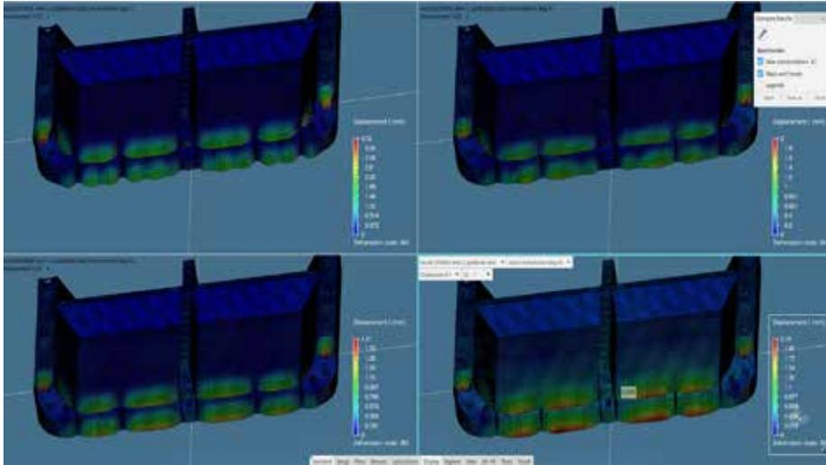
Figure 7: Displacement on section for cases 1,2,3 and 5 [7].
