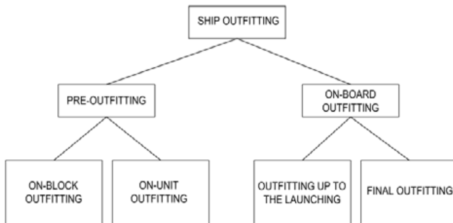
Figure 1 Breakdown structure of outfitting stages
