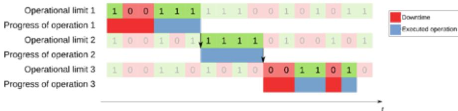
*Figure 4 Example of sequence of marine operations with weather downtime. Operations 1 and 2 are non-interruptible operations, and Operation 3 is interruptible operation. Considering the precedence relationships, Operation 1 is a coupled operation, while Operation 2 is an uncoupled operation*
