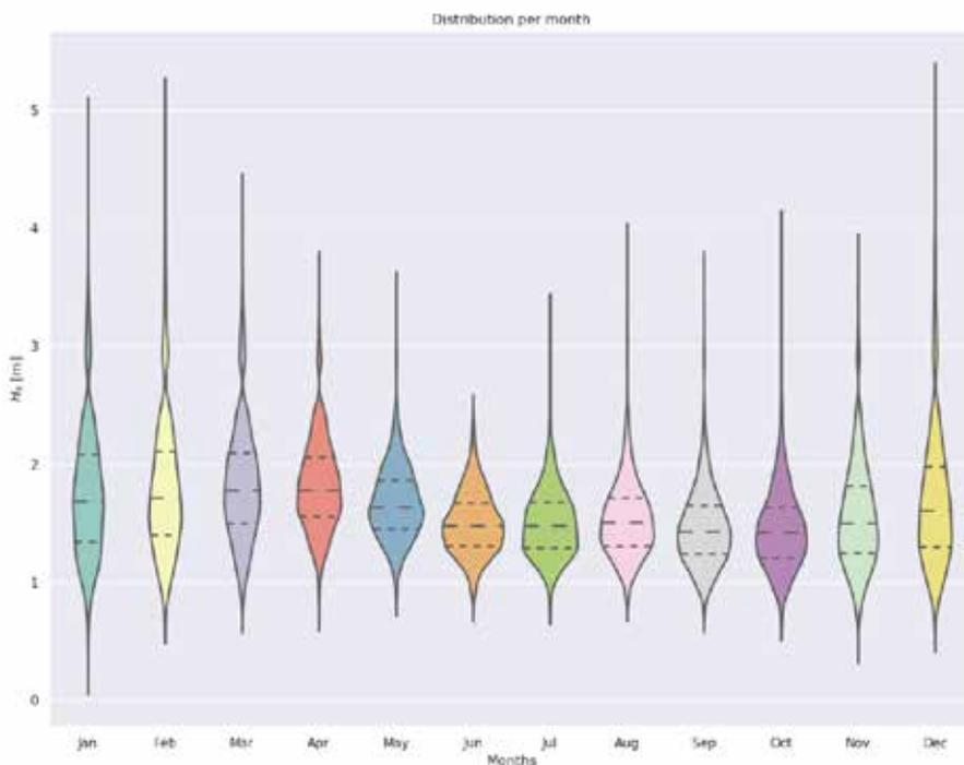
Figure 5 Example of a significant wave height distribution per month, obtained by a long hindcast time series
