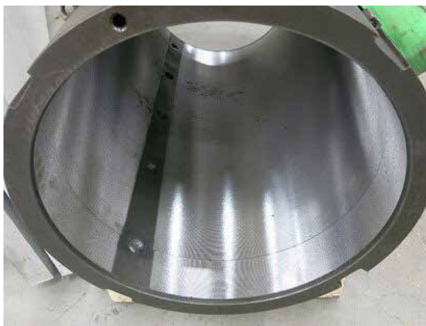
Fig. 8. Oil-lubricated stern tube bearing made of metal (source: [10])
