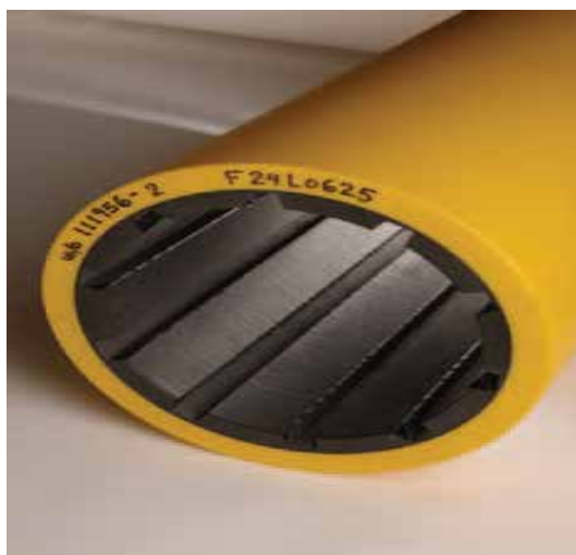
Fig. 10. Stern tube bearing lubricated with water (source: [11])
