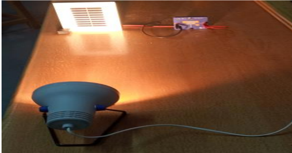
Figure 3. Experimental Setup for FS1.5 module at 200 \text{ w/m}^2 .
