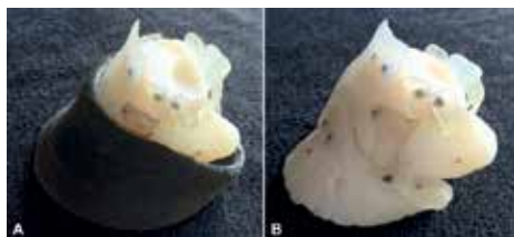
Fig. 4. The model of the equine foot printed in 3D. A, fully assembled and B, with the hoof capsule removed (Preece et al., 2013)
