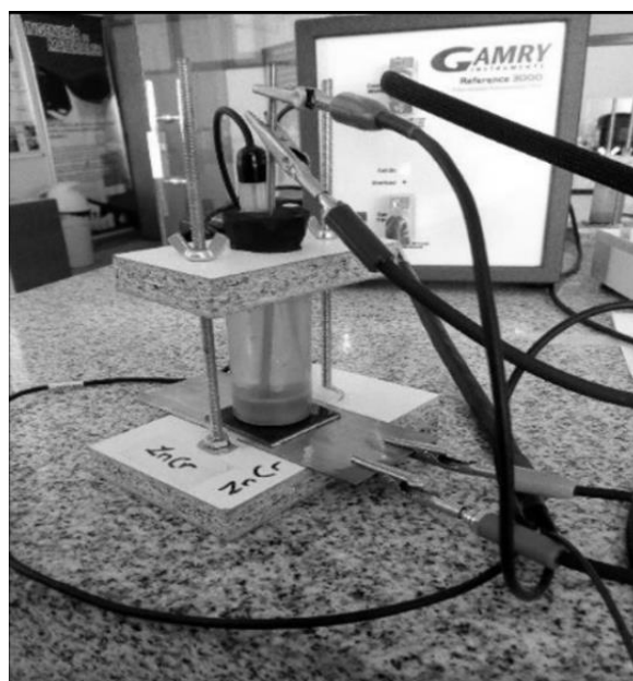
Figure 5. Arrangement of the electrochemical cell connected to Gamry 3000 equipment
