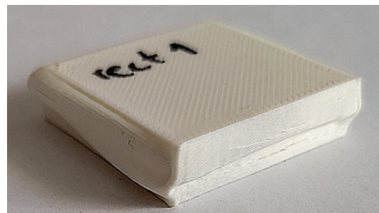
Figure 6 Compression specimen after the testing
