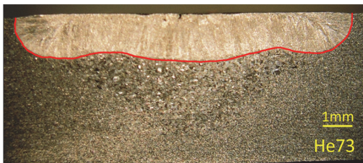
Figure 21 Typical fusion zone cross-section for purging of root side with helium and welding time of 7 seconds
