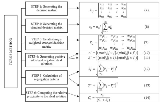
Figure 4 TOPSIS method application phases and equations
