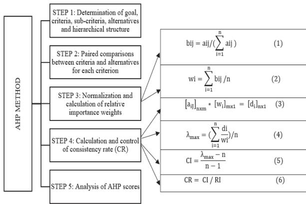
Figure 3 AHP method application steps and used equation
