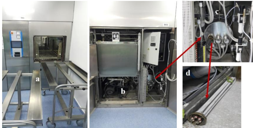
Figure 1. Horizontal steam steriliser (big autoclave): (a) outside front view; (b) inside front view; (c) steam generator; (d) resistive heating element.
