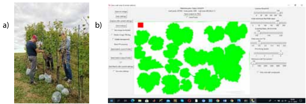
Figure 2. Manual measurement of leaf wall area a) storing each leaf in a plastic bag b) leaf wall area evaluating using software programme (Easy leaf area)
