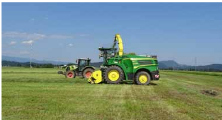
Slika 1. Samohodni silažni kombajn John Deere 8500i u radu Figure 1. John Deere 8500i self-propelled forage harvester in operation
