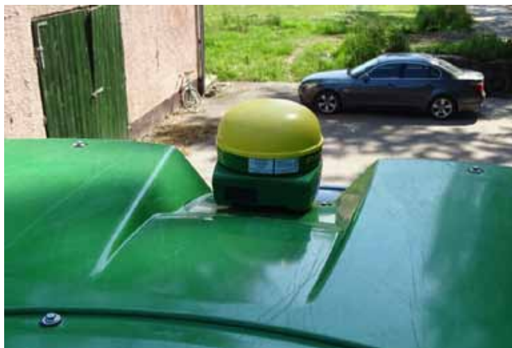
Slika 3. Satelitska antena (prijamnik) John Deere StarFire 3000 Figure 3. Satellite receiver John Deere StarFire 3000
