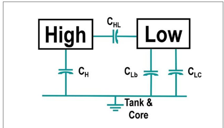
Figure 3. Dielectric circuit of a two-winding transformer showing  $C_L$  components
