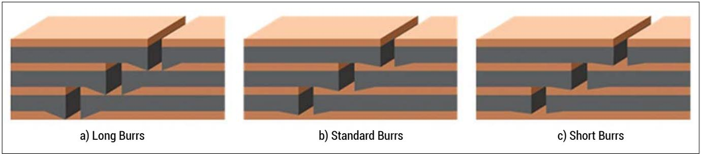
Figure 2. Expanded view of step-lapped edges of stacked cores
