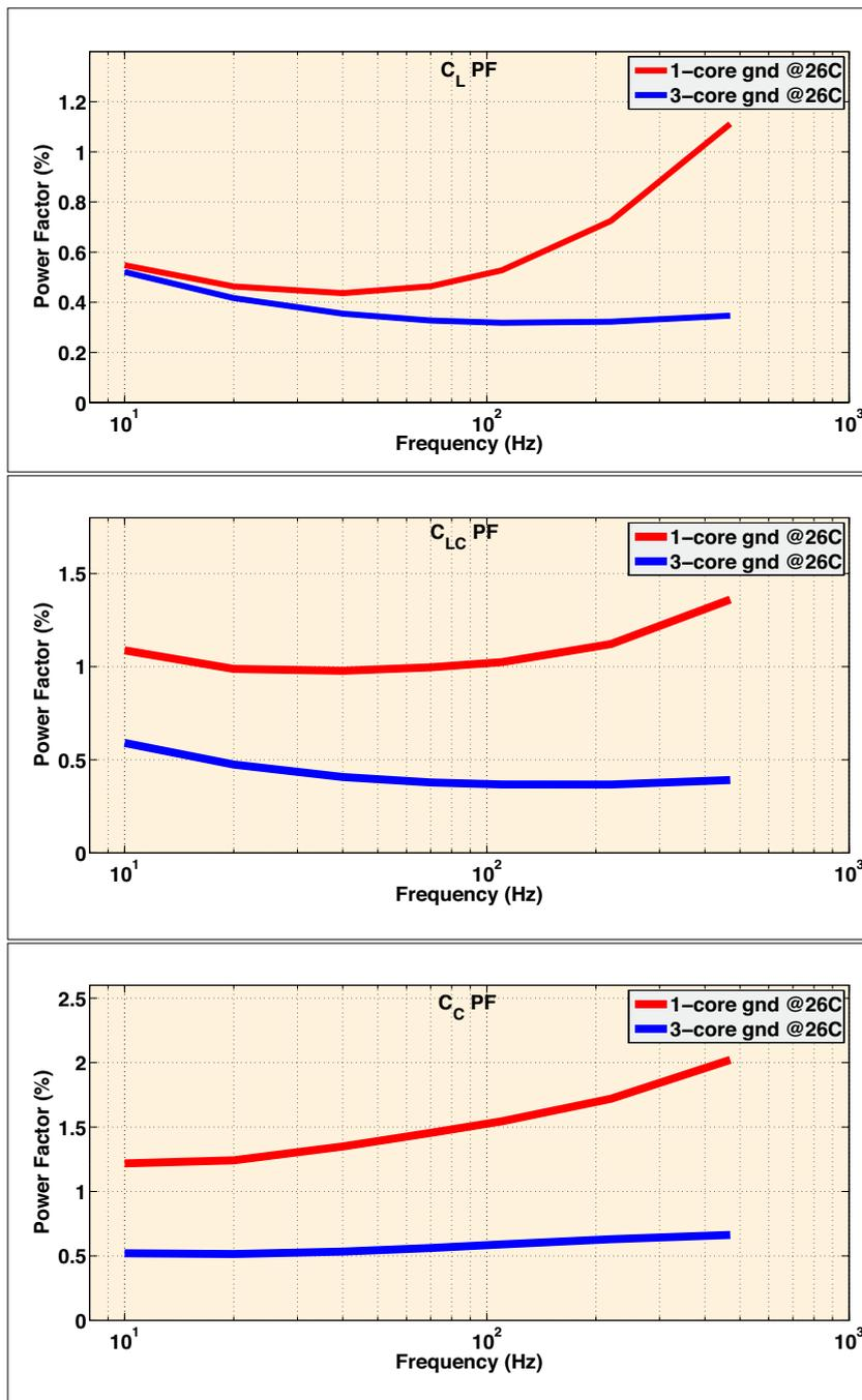
Figure 7. Case study 1 - VFPF traces on 1-core ground (high interlaminar resistance) vs. 3-core ground (low interlaminar resistance) connected on  $C_L$ ,  $C_{LC}$  and  $C_C$
