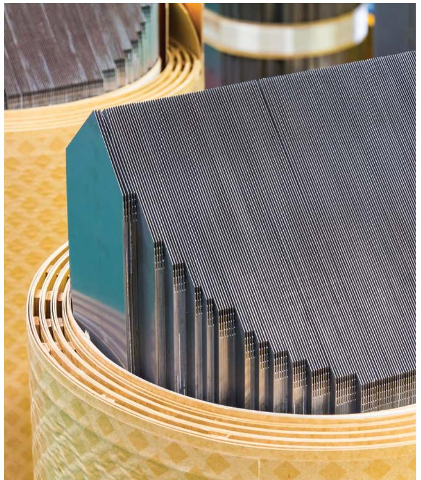
Figure 9. Transformer core detail (image shown is for illustration purposes only)
