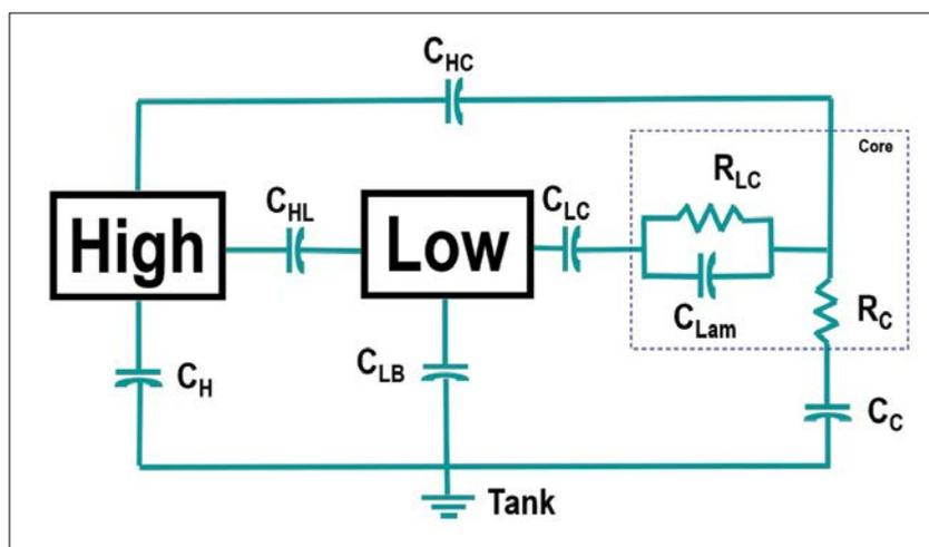
Figure 5. Dielectric circuit of a two-winding transformer showing insulations segments associated with the core
