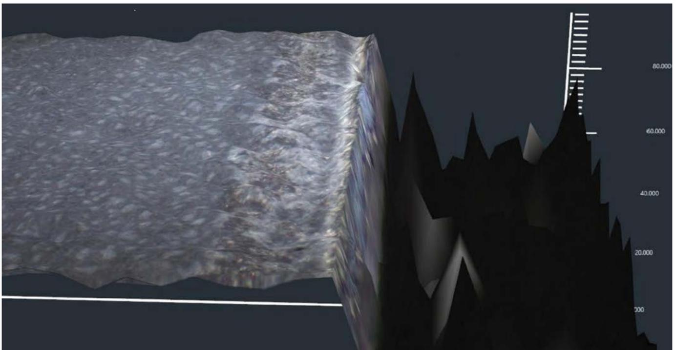
Figure 1. Microscopic view of burrs on the edge of core lamination
