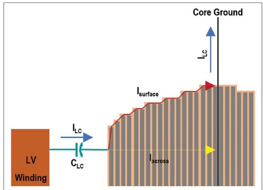
Figure 4. Current components through the core
