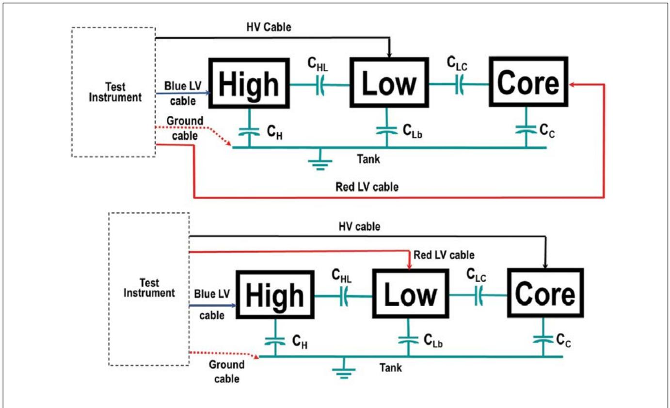
Figure 6. Setup for PF measurement on  $C_{Lb}$  and  $C_{Lc}$  (top diagram), and  $C_c$  (bottom diagram)
