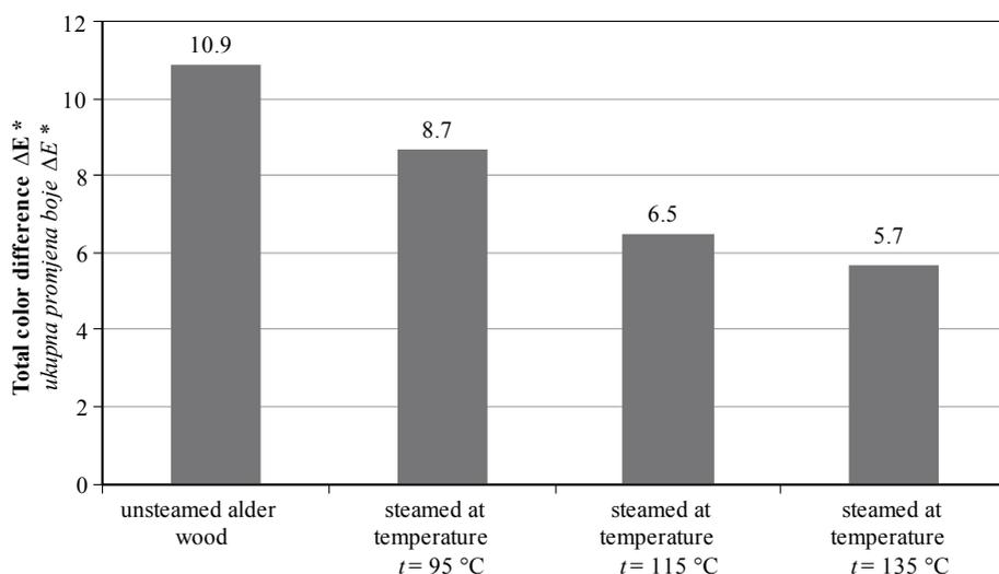
**Figure 7** Influence of UV radiation on values of total colour difference  $\Delta E^*$  of unsteamed and steamed alder wood
