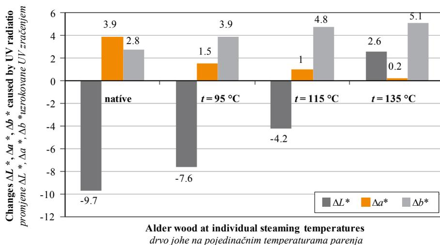
**Figure 6** Values of total changes  $\Delta L^*$ ,  $\Delta a^*$ ,  $\Delta b^*$  generated by the action of UV radiation on the surface of alder wood in Xenotest Q-SUN Xe-3-HS during 298 h irradiation
