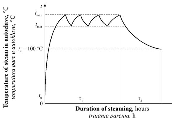
**Figure 1** Mode of colour modification of alder wood with a saturated steam-air mixture or saturated water steam
