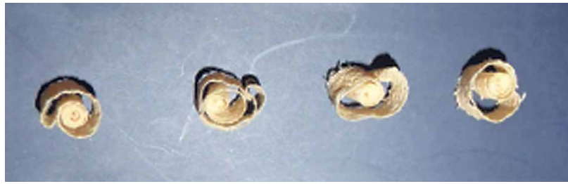
Figure 5 Exemplary collected chips from orthogonal cutting on sliding microtome in longitudinal direction to pine wood fibres; chips were created during cutting process with set uncut chip thickness h = 0.15 mm
