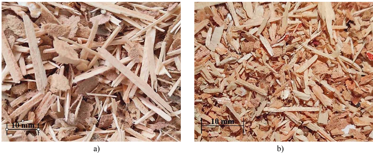
Figure 3 A particle fraction considered as useful a) particles for core layers (PCL) from 2 mm sieve, b) microparticles (MP) from 1 mm sieve
