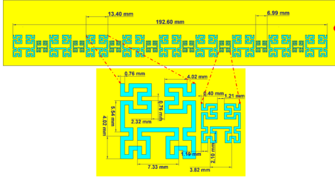
Fig. 3. The proposed MTM defect arrays.
