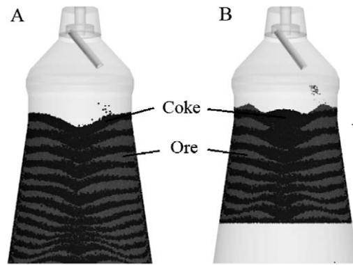
Figure 1 The vertical section views of burden distribution with non-central and central coke charging (A. non-central coke charging, B. central coke charging.)
