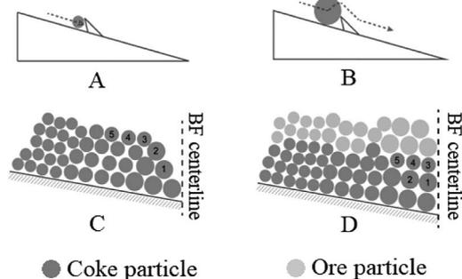
Figure 2 Schematic diagrams of coke distribution in BF with non-central coke charging (A. Motion behaviour of small coke particle; B. Motion behaviour of big particle; C. Coke distribution in surface layer; D. Coke distribution in the inner layer)
