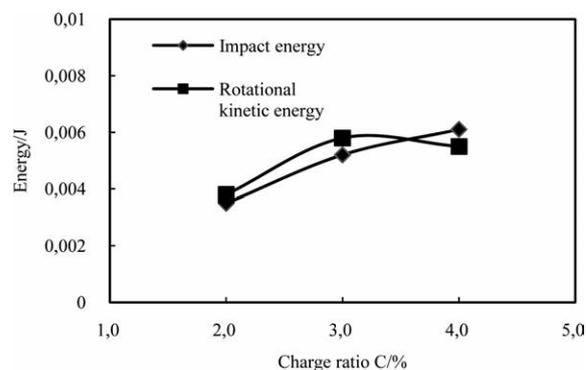
**Figure 4** Effect of the charge ratio on impact energy and rotational kinetic energy at 0,3 in  $N/N_c$
