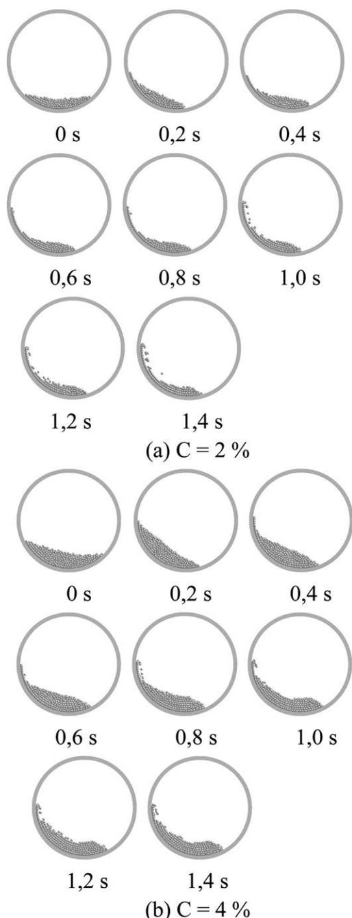
**Figure 3** Motion state of pellets at 0,3 in  $N/N_c$  for different charge ratio
