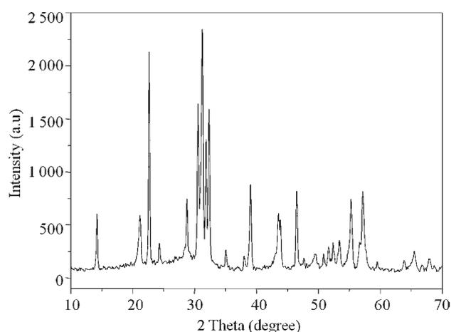
**Figure 3** XRD pattern of sample 1 of  $\text{PbTiO}_3$  nanowire.
