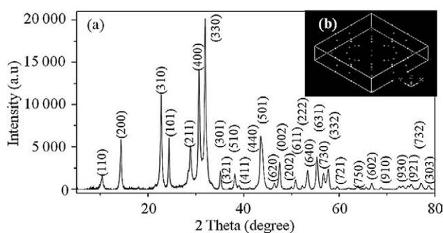
**Figure 4** Characterization of  $\text{PbTiO}_3$  new structure in sample 2 by XRD patterns.
