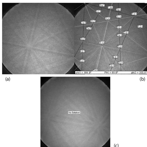
**Figure 2** Kikuchi pattern of  $\text{PbTiO}_3$  nanowire. (a) Kikuchi pattern obtained from the collection of the crystal grains as seen in Figure 1(b). (b) Kikuchi pattern calibrated in Figure (a). (c) Kikuchi pattern with unknown data.
